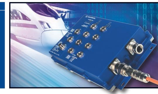
With the new Fiber-optic OCTOPUS OS20 and OS30 Switches Hirschmann<sup>™</sup> now also offers IP67-Compliant Gigabit Ethernet Functionality, thus Setting a further Milestone for Powerful Switches in Harsh industrial Environments.
